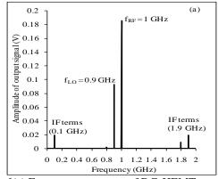
Fig. 6(a) Frequency spectrum of DG-HEMT as mixer
