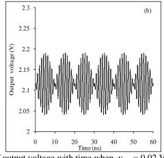
Fig. 5(b) Variation of output voltage with time when  $v_{LO} = 0.02$  V;  $V_{ds} = 1$  V,  $V_{gs2} = 0$  V.
