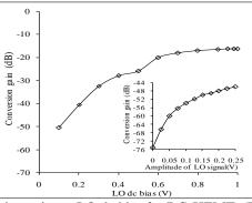
Fig. 7 Variation of conversion gain vs. LO dc bias for DG-HEMT, (Inset) variation of Conversion Gain vs. LO dc bias for double gate MOSFET RF mixer [15]
