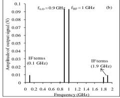
Fig. 6(b) Frequency spectrum of DG-HEMT as mixer application when  $V_{gs2} = -0.1 V$
