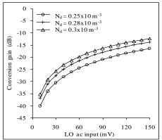
Fig. 8 Variation of conversion gain with LO ac input  $(v_{\rm LO})$  for different value of donor layer doping concentration  $(N_d)$
