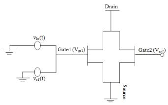
Fig.3. Schematic of proposed DG-HEMT mixer
