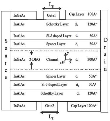
Fig. 1 Double-gate InAlAs/InGaAs/InAlAs structure HEMT [9-10]
