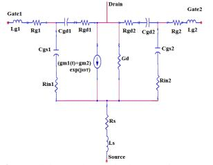
Fig. 4(b) Small signal equivalent circuit (SSEC) for DG-HEMT
