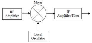
Fig. 2 Block diagram of mixer used in communication receiving system
